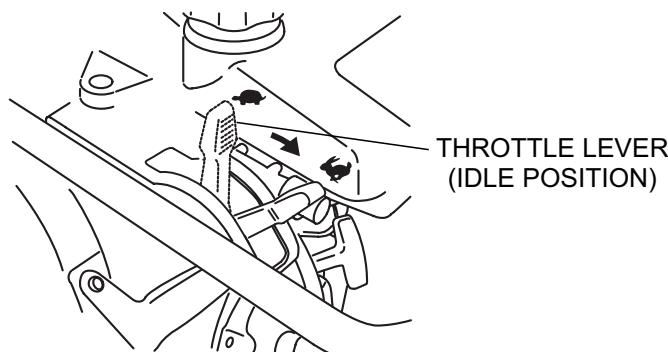
Figure 6. Throttle Lever (Idle Position)
