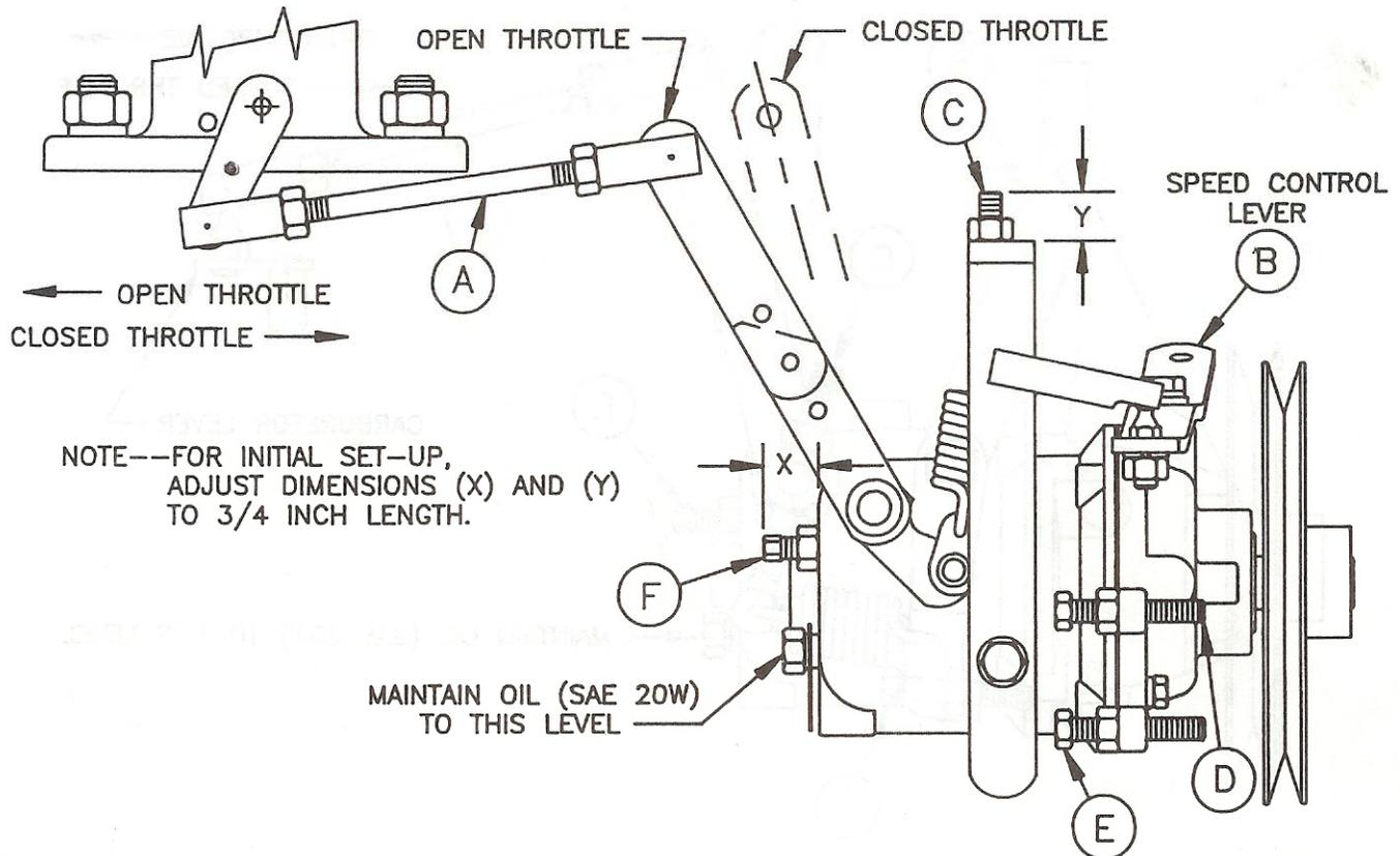
1. MOVE SPEED LEVER (B) TO PUT SPRING TENSION ON GOVERNOR AND ADJUST THROTTLE ROD (A) TO GIVE ABOUT 1/16 INCH CLEARANCE BETWEEN CARBURETOR LEVER AND WIDE-OPEN STOP ON CARBURETOR.
