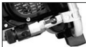
water supply opened (valve lever parallel)
