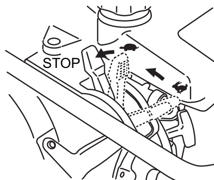
Figure 11. Throttle Lever (Stop Position)
