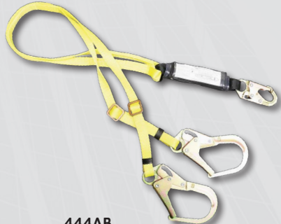
444AB #Z74 locking snaphook one end #Z136 snaphooks (2 1/2" opening) other two ends Pack style shock absorber Adjustable length
