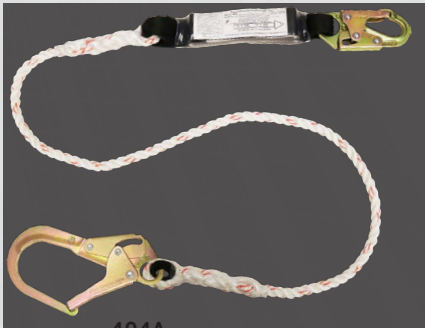
404A #Z74 locking snaphook one end #Z136 snaphook (2 1/2" opening) other end Pack style shock absorber
