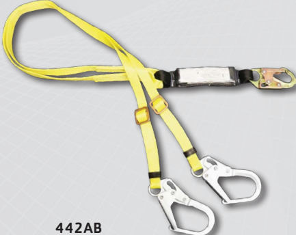
442AB #Z74 locking snaphook one end #69 snaphooks (1 3/4" opening) other two ends Pack style shock absorber Adjustable length
