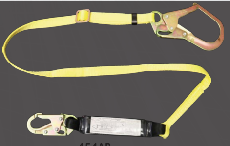
454AB #Z74 locking snaphook on one end #Z136 snaphook (2 1/2" opening) other end Pack style shock absorber Adjustable length
