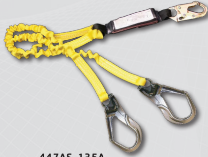
447AS-135A #Z74 locking snaphook one end #135A aluminum snaphooks (2 1/2" opening) other two ends Pack style shock absorber with elastic stretch
