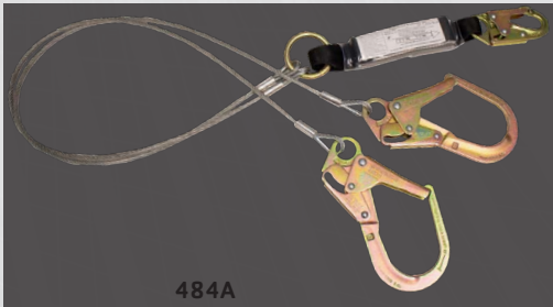
484A #Z74 locking snaphook one end #Z136 snaphooks (2 1/2" opening) other two ends Pack style shock absorber
