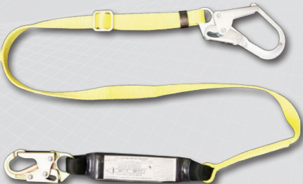
452AB #Z74 locking snaphook on one end #69 snaphook (1 3/4" opening) other end Pack style shock absorber Adjustable length
