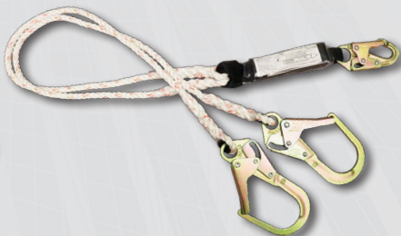
434A #Z74 locking snaphook one end #Z136 snaphooks (2 1/2" opening) other two ends Pack style shock absorber
