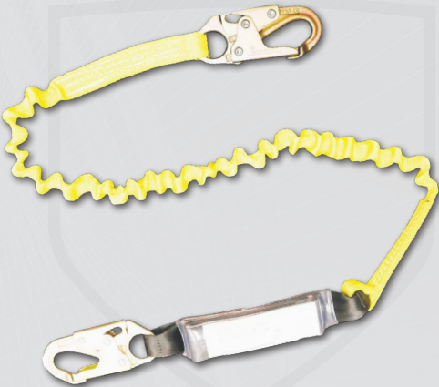
♦♦ 450AS #Z74 locking snaphooks on each end Pack style shock absorber with elastic stretch
