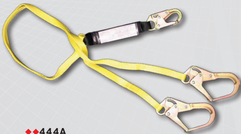
♦♦ 444A #Z74 locking snaphook one end #Z136 snaphooks (2 1/2" opening) other two ends Pack style shock absorber
