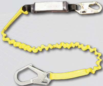
452AS #Z74 locking snaphook one end #69 snaphook ( 1 3/4" opening) other end Pack style shock absorber with elastic stretch
