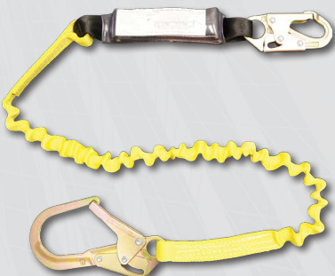
454AS #Z74 locking snaphook one end #Z136 snap (2 1/2" opening) other end Pack style shock absorber with elastic stretch
