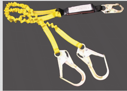
♦♦ 444ASZ #Z74 locking snaphook one end #Z136 snaphooks (2 1/2" opening) other two ends Pack style shock absorber with elastic stretch
